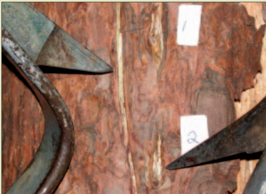
Marks on section of trunk from a goshawk-nesting tree compared with tree climbing irons belonging to a suspect. M Thomas (RSPB)
